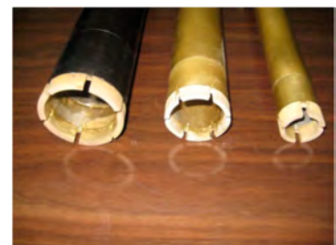
<암석 NX,BX,25 mm Core Bit x 300mm>
