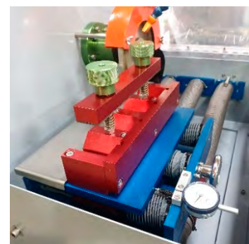
< A four-sample fixing device and precise left-right feed system >
