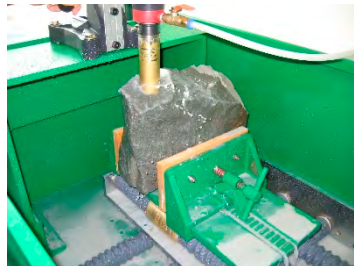
<Rock core drilling >
