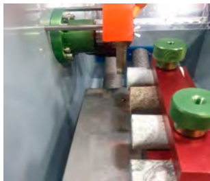
< Simultaneous grinding of four rock cores or graphite rods >
